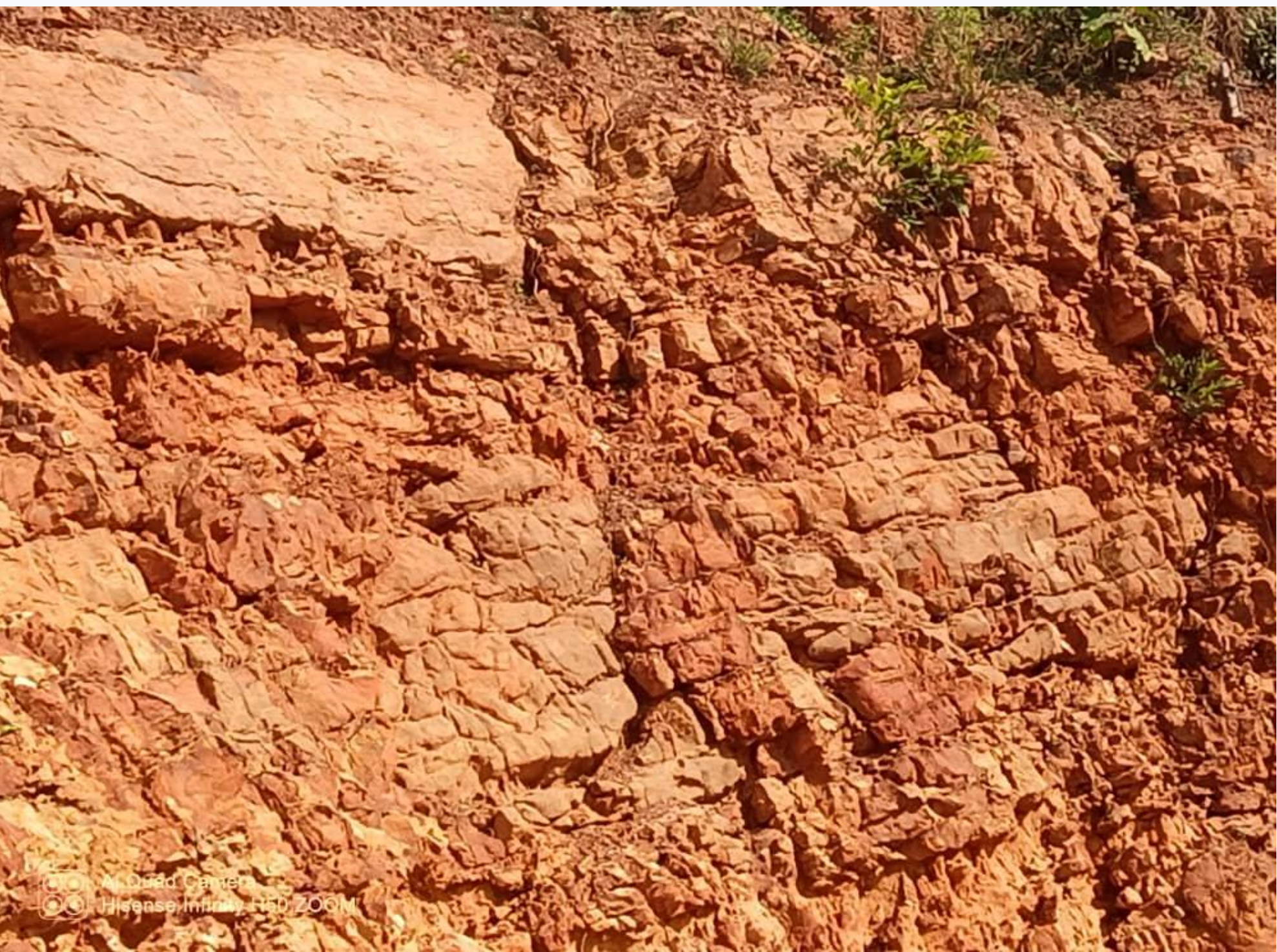
Fig. 4: Weathered, jointed basement outcrop within the study corridor, showing intense fracturing consistent with reactivated Precambrian shear zones.
